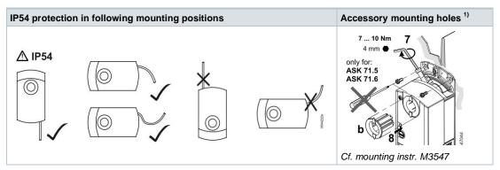
Not to be used for fixation of the actuator, use anti-rotation-bracket instead.
