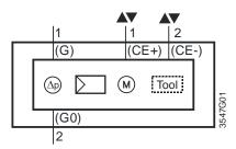
Tool = Configuration and maintenance interface (Series E and later: 7-pin connector)
